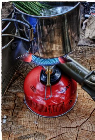
A canister of the hydrocarbon named propane provides fuel for this camp stove.
