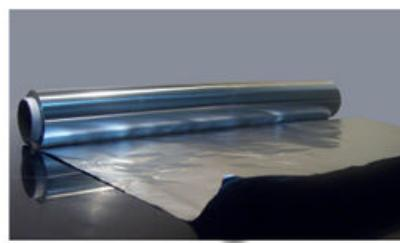
Most metals are malleable. This means they can be formed into thin sheets without breaking, like this foil made of the metal aluminum (Al).
