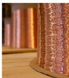
Most metals are ductile. This means they can be pulled into long thin shapes, like these wires made of the metal copper (Cu).
